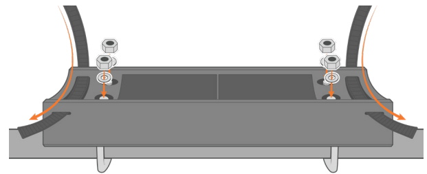
Figure 3: Tighten the clamp to the instrument cage.
