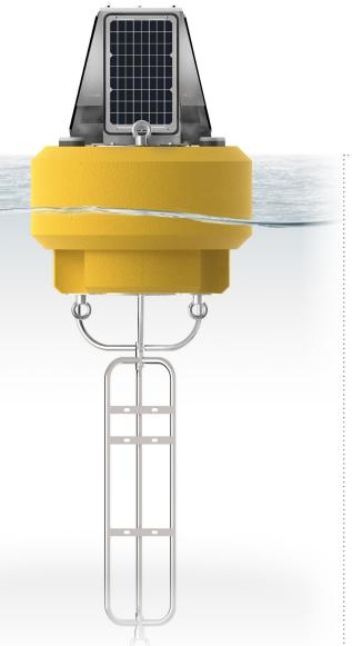
The NexSens CB-250 Data Buoy is designed for deployment in lakes, rivers, coastal waters, harbors, estuaries and other freshwater or marine environments. The floating platform supports both topside and subsurface environmental monitoring sensors including weather stations, wave sensors, thermistor strings, multi-parameter sondes, Doppler current profilers and other monitoring instruments.
