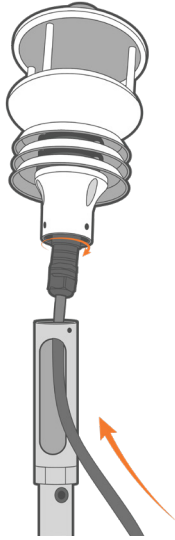
Figure 4: Connect the MaxiMet sensor cable.
