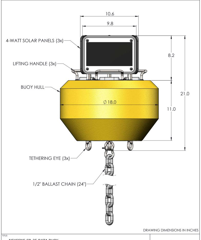
NEXSENS CB-25 DATA BUOY
